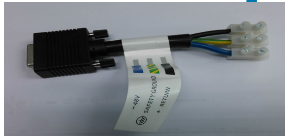
Figure 4-6: Connecting -48V DC Power Cable Adapter
