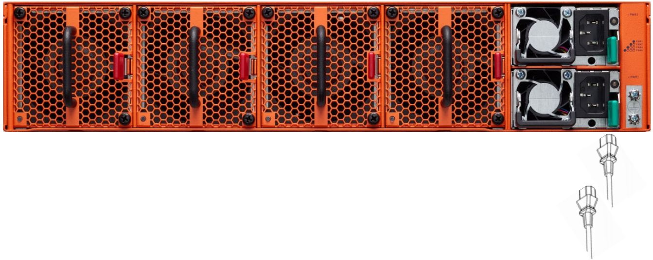
Figure 4-5: Connecting AC Power on a GigaVUE-TA200
