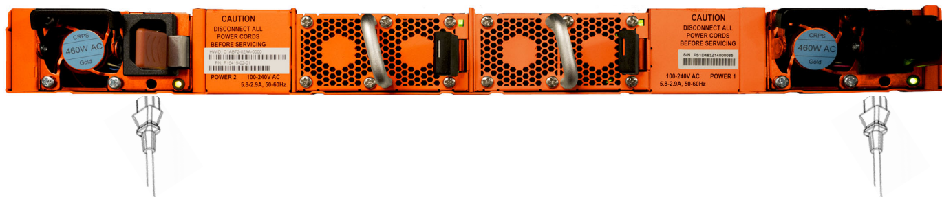
Figure 4-3: Connecting AC Power
