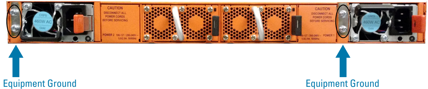
Figure 4-1: Ground Screws (GigaVUE-TA10 Shown)
